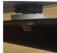
Mounts on rubber grommets to stop vibration
